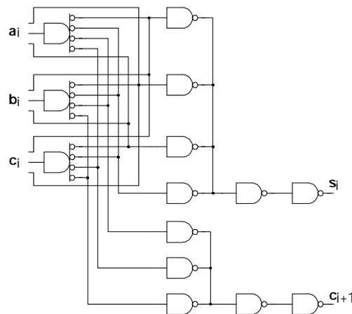
Fig. 12. Example of one-bit adder circuit
