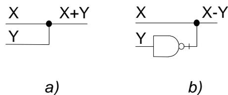
Fig. 11. The example schemes for realizing addition and subtraction operations in current-mode basis.
