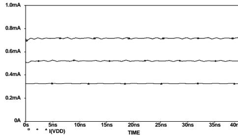
Fig. 6. Supply current  $I(VDD)$  feeding oscillator: (a) classical inverters, (b) current-mode gates
