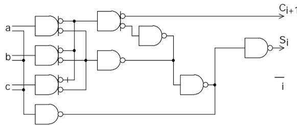
Fig. 14. The 9-th gates version of one-bit adder
