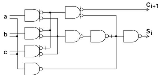
Fig. 15. The 8-th gates version of one-bit adder
