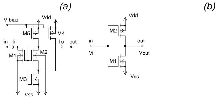
Fig. 2. Current-mode CMOS digital gate (a) and classical, voltage CMOS inverter (b)
