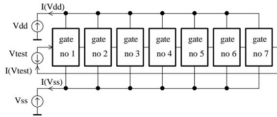
Fig. 4. Ring oscillator composed of seven gates
