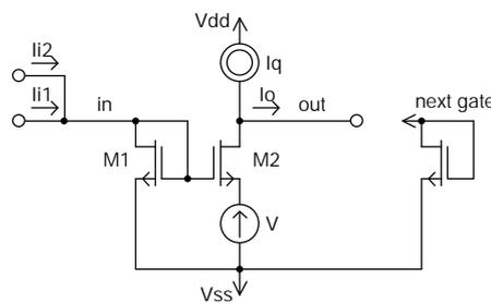
Fig. 1. Concept of current-mode gate
