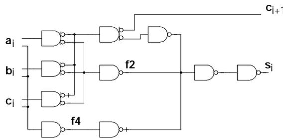
Fig.13. The 10-th gates version of one-bit adder
